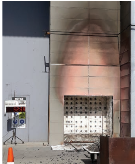
Territory panels intact following removal of fire crib.
